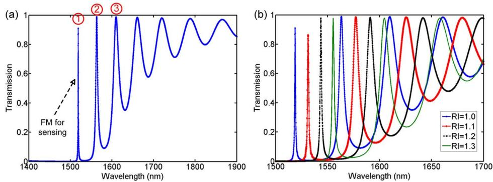
Fig. 4. (a) 3-D-FDTD transmission spectrum of the proposed 1-D PC-NCS device. (b) Composed transmission spectra of the proposed 1-D PC-NCS as a function of RI changed from RI = 1.0 to RI = 1.3.
