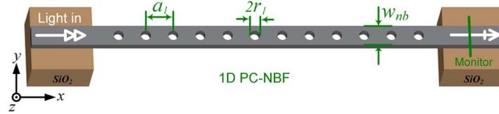
Fig. 1. Schematics of the single silicon 1-D PC nanobeam bandgap filter (1-D PC-NBF). The radius of air-hole gratings are kept in same as  $r_1 = 90$  nm. The structure is symmetric with respect to its center. Periodicity  $a_1 = 390$  nm is the center-to-center distance between the gratings;  $w_{nb} = 700$  nm is the width of the 1-D PC nanobeam waveguide. The thickness of the silicon ridge waveguide is 220 nm.  $n_{si} = 3.46$ , and  $n_{air} = 1.0$ .
