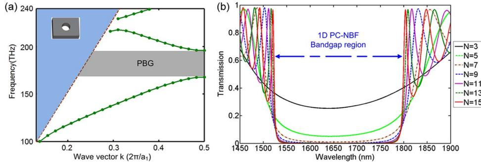
Fig. 2. (a) TE band diagram of the single 1-D PC nanobeam waveguide with  $r_1 = 90$  nm,  $w_{nb} = 700$  nm, and  $a_1 = 390$  nm. The thickness of the nanobeam waveguide is 220 nm. (Inset) Unit cell of waveguide used in the band structure calculation. (b) Transmission spectra obtained by using 3-D-FDTD calculation for different grating number ( $N$ ), while other structure parameters keep fixed.
